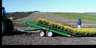
The Drop Trailer allows a full load of containerized plants to fill the bed of the trailer and then be transported to another location. By simply dropping the back end of the trailer, the containers full of plants easily off-load on to the ground in just seconds.
