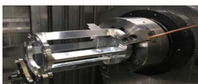
DMG MORI CTX BETA 1250TC MILL TURN 5 axis and 60" bar feeder X: 17.7"/450mm Y: 3.94"/100mm Z: 51.2"/1,301mm
